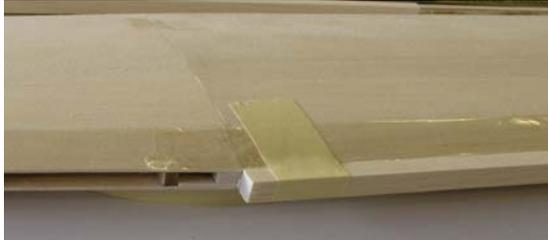
17. Glue 0.8mm ply end ribs to balsa tips. Again there is a Left & Right! Roughly shape and glue tip in place taking care to align tip end rib with wing end rib.
