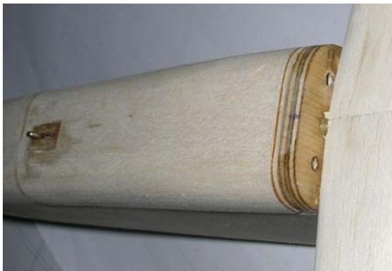
27. Fit and hold wing in position and drill hole for wing retaining dowel brass tube (use drill described on plan). Drill a pilot hole first using a long 3mm piano wire drill.
