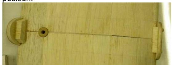
46. Fit wing fairing ply alignment plates and balsa supports.
