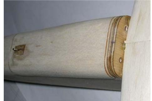
35. Drill Hatch dowel locating hole in fuselage.
