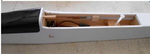
31. Fit Elevator servo. Mount On/Off switch. Fit Rudder servo.
