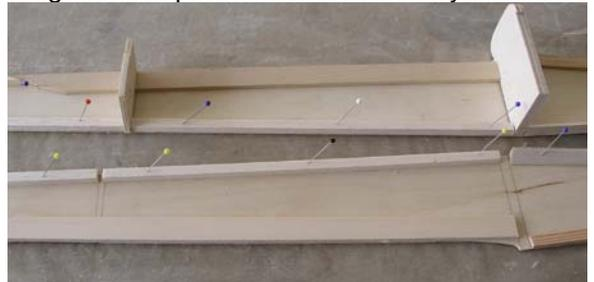
5. Glue strip longeron super structure including 6mm tail-seat to fuselage sides.
