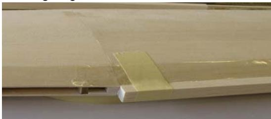
16. Glue 0.8mm ply ends to centre section TE, again not letting any glue contact torque rods.
