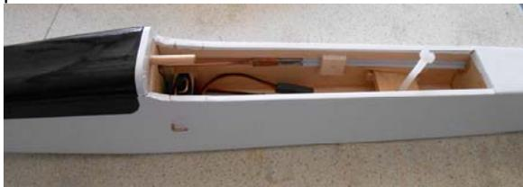
31. Fit Elevator servo. Mount On/Off switch. Fit Rudder servo.
