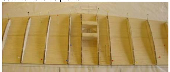
8. Cut 2mm sub-rib to length and glue in position.
