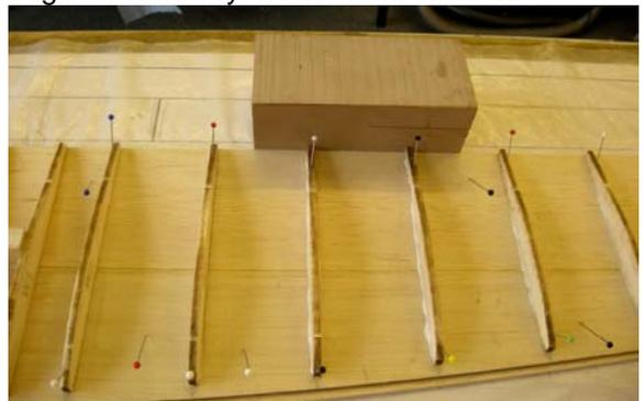
5. Elevate front of underside of bottom sheeting with scrap 1.5mm balsa to conform with contour at front of Wing rib (see plan)
