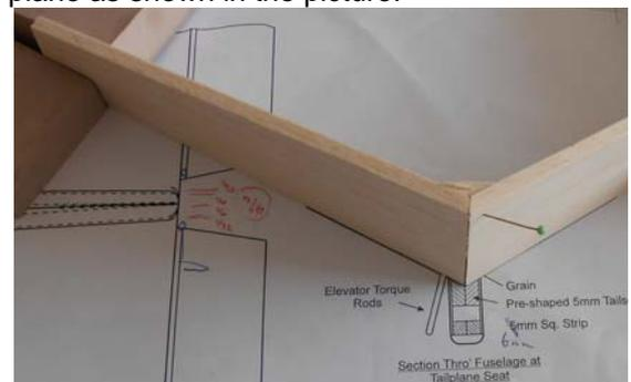
13. Place fuselage on flat surface with weights to hold it in position.
