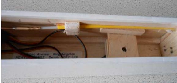
14. Fit Fuselage bottom front and back plus 10mm top nose sheet.
